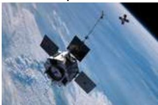
**Left:** The identical Radiation Belt Storm Probes will follow similar orbits that will take them through both the inner and outer radiation belts. The highly elliptical orbits range from a minimum altitude of approximately 373 miles to a maximum altitude of approximately 23,000 miles.
