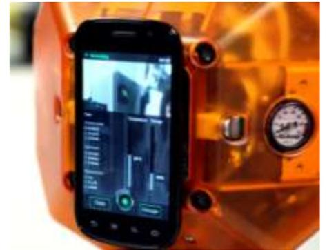
*The Nexus S runs an app that records activity on the gyroscope, accelerometer, and 3D compass.*
