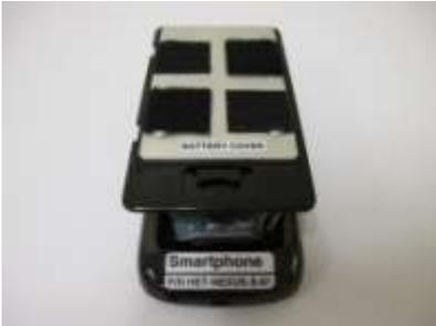
Micire also had to figure out how to power up the phone without using a lithium-ion battery pack. "Getting a lithium-ion battery certified for the station was going to probably be greater than two years," he explained. Alkaline batteries had already been approved for space travel because they degrade "more nicely." Rather than explode and catch on fire, alkaline batteries will instead leak electrolyte fluid, which is easier to contain. The team on the
