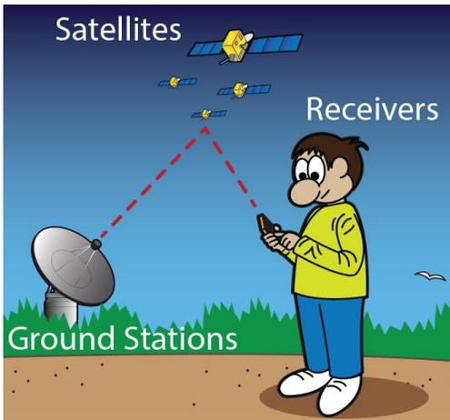
*The Global Positioning System (GPS) is made up of satellites, ground stations, and receivers.*
