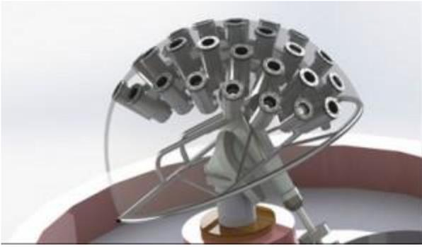
Evryscope contains 27 61-mm telescopes fitted onto a single German Equatorial mount. The instrument will take a continuous movie of the night sky, collecting data in 2-minute exposures, starting later this year. *J. Ratzloff / N. Law / UNC Chapel Hill*
