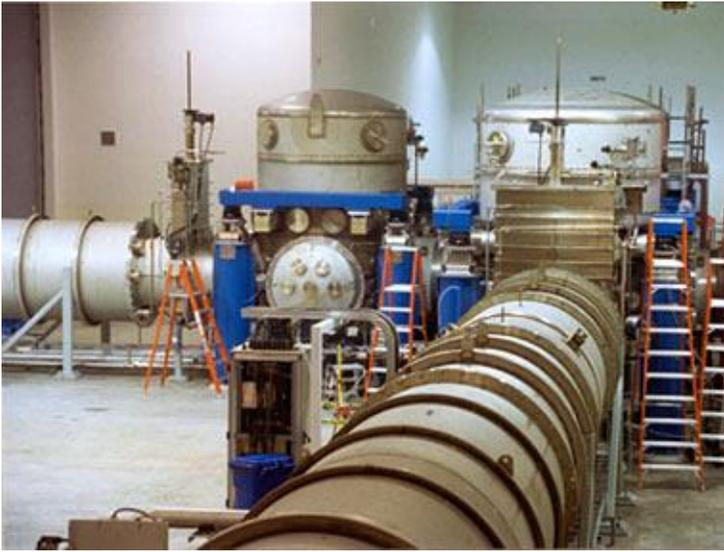
The meeting of the arms. The light pipes and the equipment in their ends (seen here) are kept in an ultrahigh vacuum. *LIGO Laboratory*.
