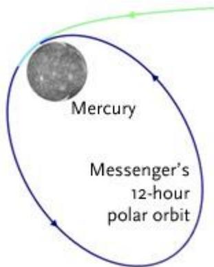
Messenger's initial polar orbit around Mercury ranged in altitude from just 120 miles (200 km) to about 10,000 miles (15,000 km). Later the orbit was adjusted so the spacecraft passed even closer.
