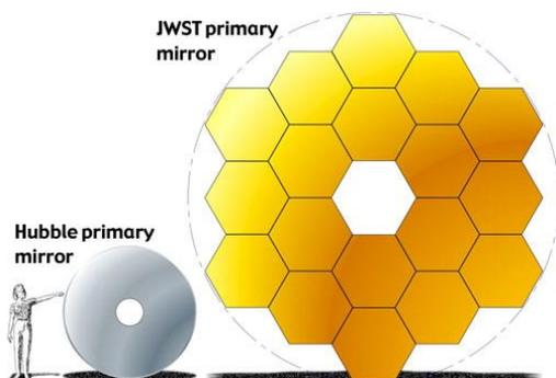
A comparison of the primary mirror on the Hubble Space Telescope versus the James Webb Space Telescope. NASA
