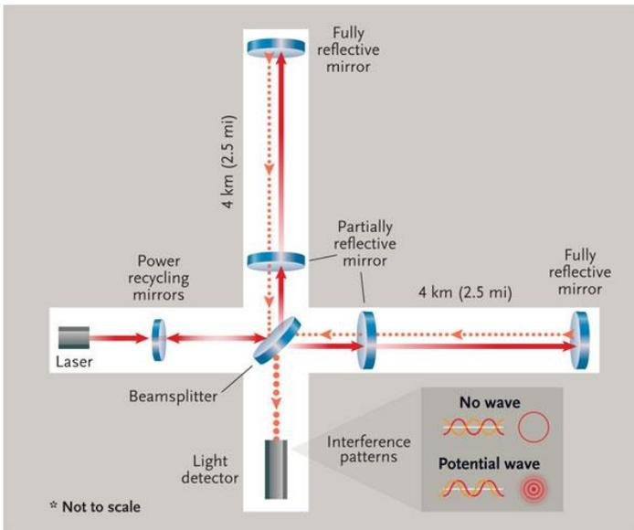
In this schematic of LIGO, a beamsplitter sends light along two paths perpendicular to each other. Each beam bounces between two mirrors, one of which allows a fraction of the light through. When the two transmitted beams meet and interfere, they'll cancel each other out — if the length of the path they've each traveled has remained constant. But if a gravitational wave passes through, it'll warp spacetime and change that distance, creating an interference pattern. S&T: *Leah Tiscione*
