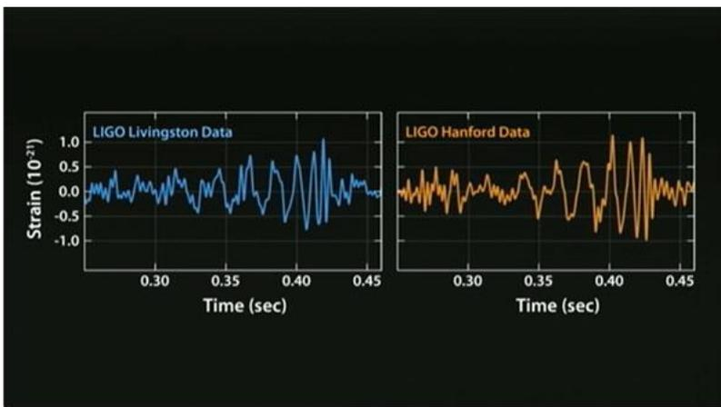
These are the actual gravitational waves detected by LIGO, first at Livingston then a fraction of a second later, in the Hanford detector. *LIGO*
