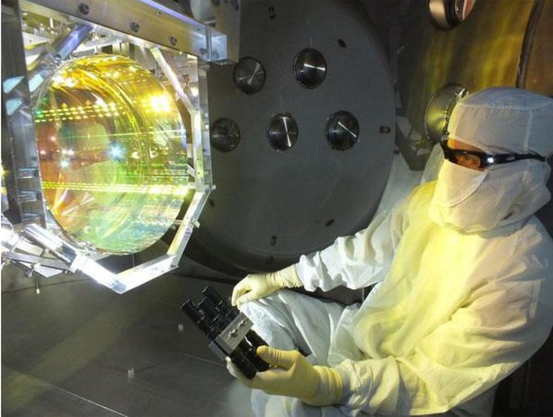
A LIGO technician checks the detector's optics for contaminants by illuminating its mirrors. *LIGO*
