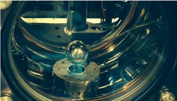
This photo shows the experimental set-up, with the 25-mm-diameter sphere at the center of the vacuum chamber. The experiment measures the force between the sphere and cesium atoms (not visible). *Holger Mueller*
