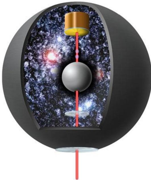
An artist's impression shows the aluminum sphere of the experiment, the Cesium atoms (violet dots), and the laser beam that travels from one of the sphere to the other every time it flashes. *Simca Bouma*
