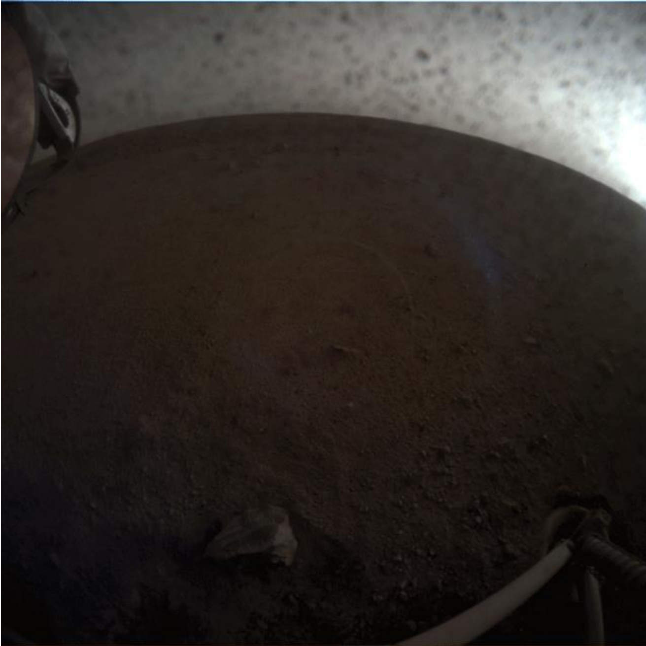
A fish-eye view of NASA's InSight lander deploying its first instrument onto the surface of Mars, taken by the spacecraft's Instrument Context Camera (ICC) on Dec. 19, 2018. Image Credit: NASA/JPL-Caltech
