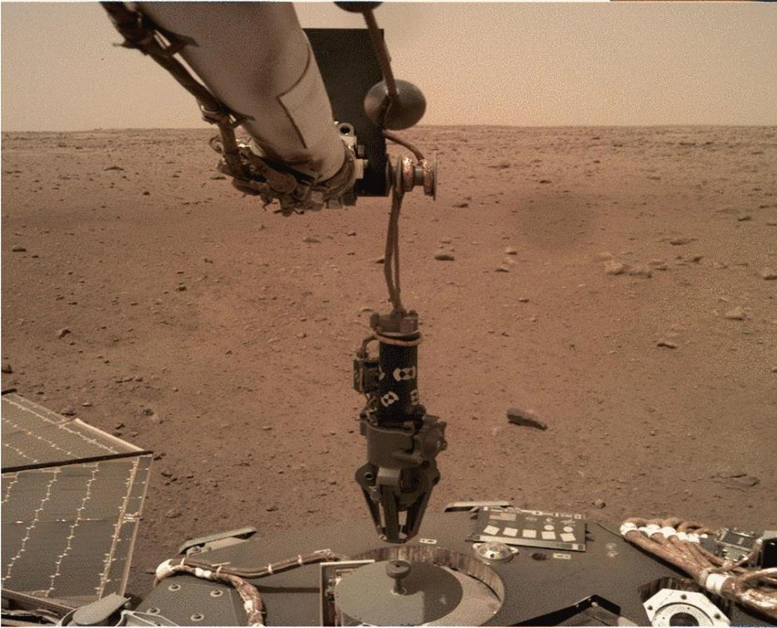
**A timelapse showing the deployment of the HP<sup>3</sup> package on the surface of Mars.**
