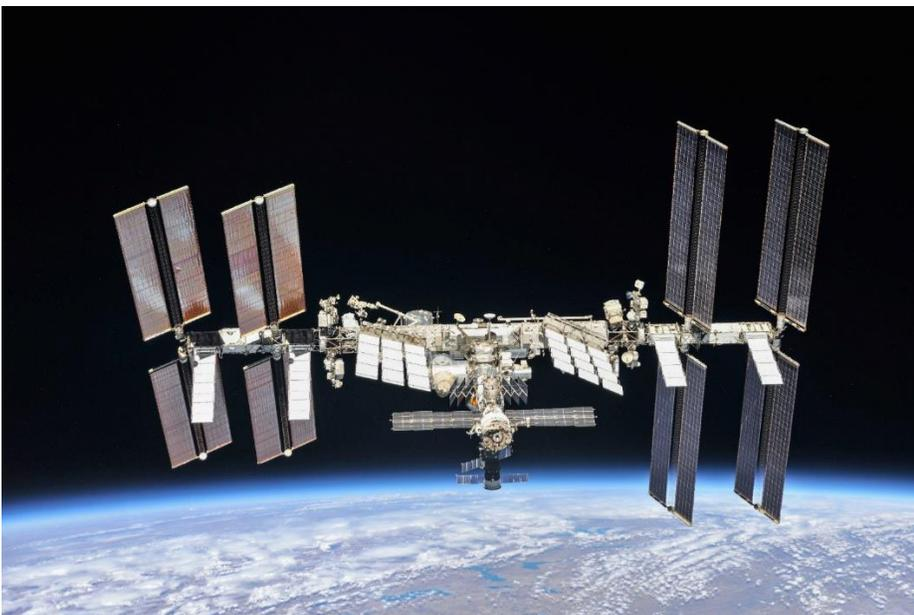
***A complete view of the ISS as of October 4, 2018, taken from the Soyuz capsule of the departing crew of Expedition 56 from their Soyuz capsule. This structure was built by materials launched into orbit by 37 United States Space Shuttle missions and 5 Russian Proton and Soyuz rockets, and assembled and maintained by 230 spacewalks, with more to come! Credit: NASA/Roscosmos More info: [bit.ly/issbasics](https://bit.ly/issbasics)***
